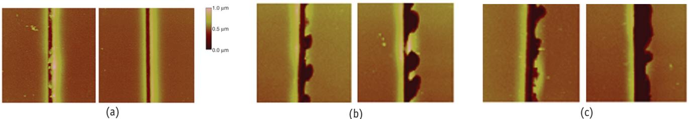
Figure 12—Two groups for a total of 20 scratches; each of them was 1000  $\mu\text{m}$  long made under a linearly increasing force from 0 to 30 mN, in a pair of orthogonal directions, and made a matrix with a spacing of 100  $\mu\text{m}$ . An “x” mark was used to indicate the observation of the chipping at the intersections.
