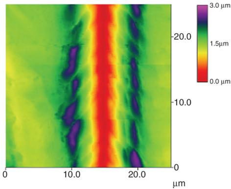
along the same trench in the applications, this test can provide a proper measurement of their mar/scratch resistance behavior in the applications; for example, the glazing material used for automobile side windows. The hard dust particles trapped between the window and the rubber seals may repeatedly mar and scratch the surface in the same trench when the window is rolled up and down.
