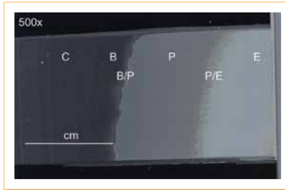
Figure 14—Cross-sectional image of an OEM automotive multi-layered paint system microtomed at magnification 500x.
