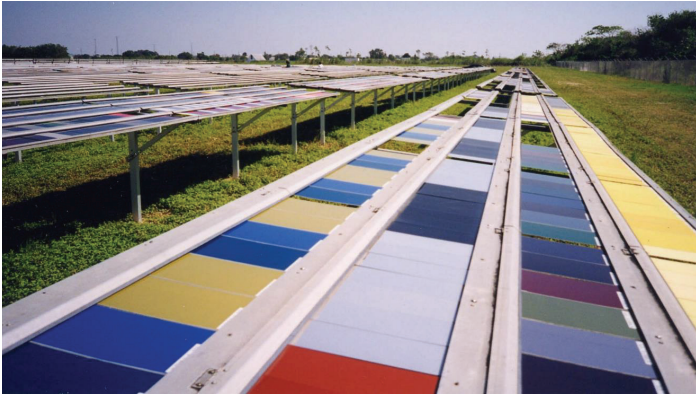
FIGURE 2—Painted panels in exposure racks in south Florida. (Upper) automotive coatings exposed at 5° south, and (lower) architectural coatings exposed at 90° south.
