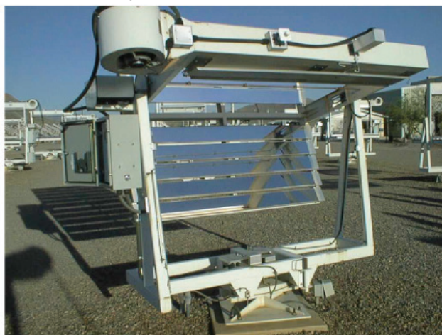
FIGURE 7—Fresnel-type accelerated outdoor exposure device.
